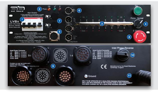
1. An input MCB provides protection against output overload faults. The MCB is rated at 32A with D characteristic providing 10 - 20 times normal rating for start-up surges.
